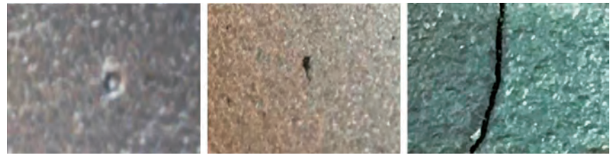
(a)气孔 (b) 缩孔 (c) 裂纹
