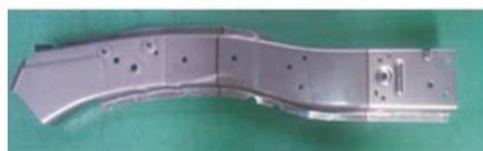
EC8激光拼焊机舱纵梁
